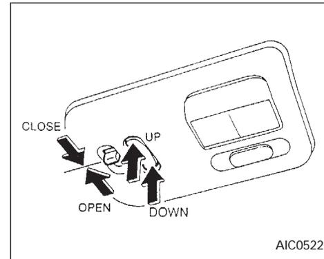
The sunroof only operates when the ignition key is in the ON position.
