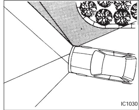
The cornering light provides additional illumination toward the turning direction. The light on the turning direction side comes on when a turn is signaled with the headlights on.
