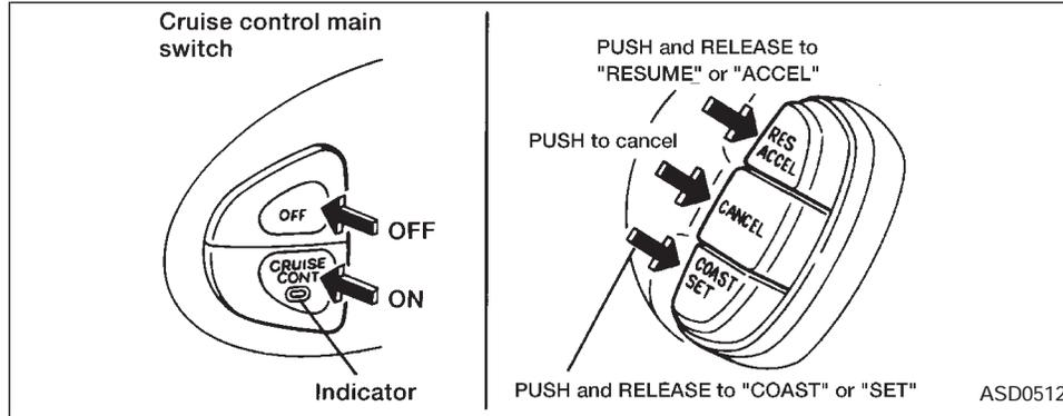
The cruise control allows driving at a speed between 30 to 90 MPH (48 to 144 km/h) without keeping your foot on the accelerator pedal.
