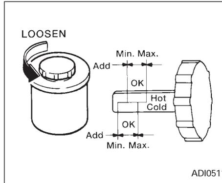
Check the fluid level in the reservoir.
