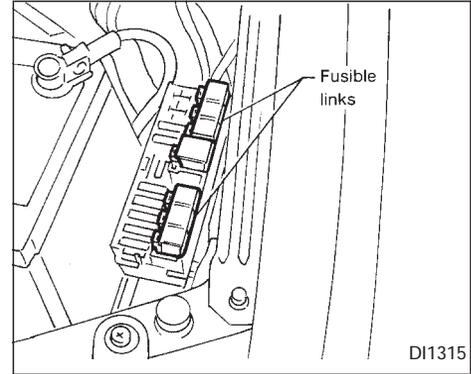
If the electrical equipment does not operate and fuses are in good condition, check the fusible links. If any of these fusible links are melted, replace only with genuine NISSAN parts.
