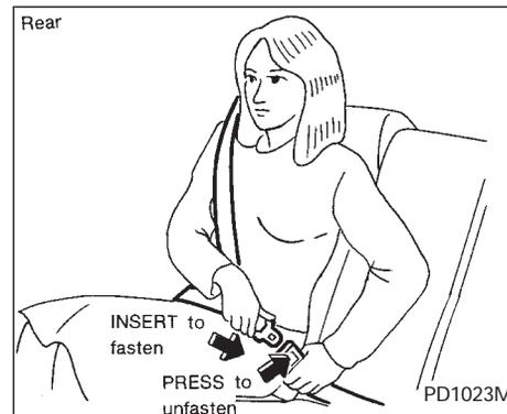
2. Slowly pull the seat belt out of the retractor and insert the tongue into the buckle until it snaps.
