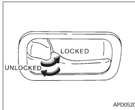
To lock a door from inside the vehicle, press the lock knob (located above the door handle) until it is flush with the door panel. To unlock, pull the lock knob to its outer position.
