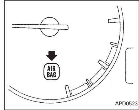
The supplemental air bag warning light, displaying AIR BAG in the instrument panel, monitors the circuits of the supplemental air bag. The circuits monitored by the supplemental air bag light are the diagnosis sensor unit, supplemental air bag modules and all related wiring.
