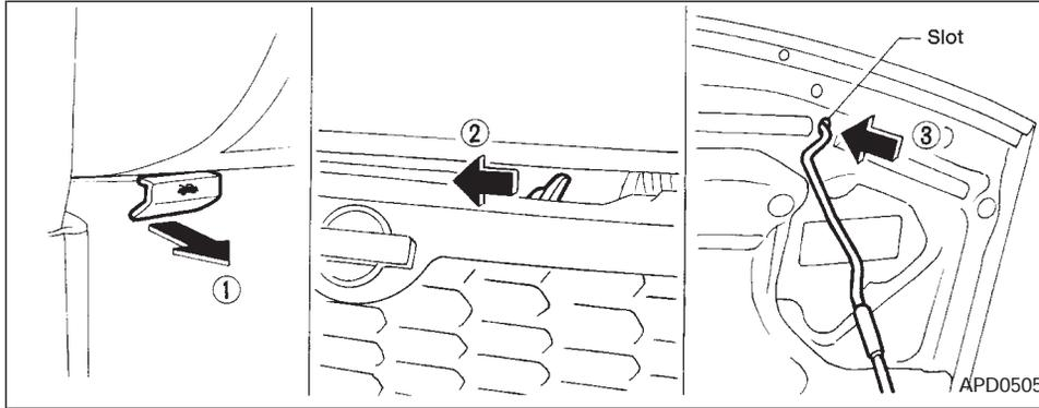
1. Pull the hood lock release handle ① located below the instrument panel; the hood springs up slightly.
