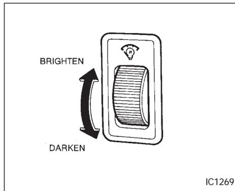
The instrument brightness control operates when the light switch is in the  $\text{☰}$  or  $\text{☷}$  position.
