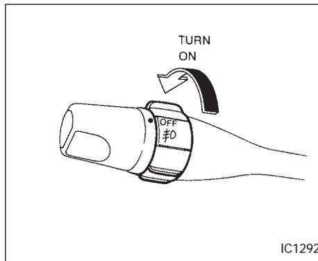
To turn the front fog lights on, rotate the switch to the  $\text{☷}$  position.
