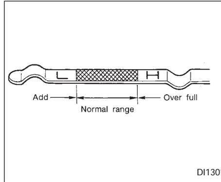
5. Remove the dipstick again and check the oil level. It should be between the H and L marks. If the oil level is below the L mark, remove the oil filler cap and pour recommended oil through the opening. **Do not overfill.**
