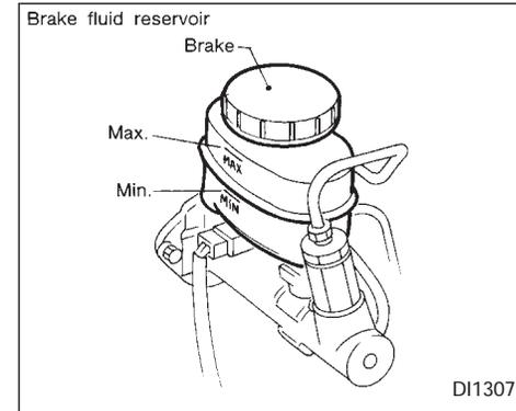
Check the brake fluid level in the reservoir. If the fluid level is below the MIN line or the brake warning light comes on, add **DOT 3** fluid up to the MAX line. If fluid must be added frequently, the system should be thoroughly checked by your NISSAN dealer.
