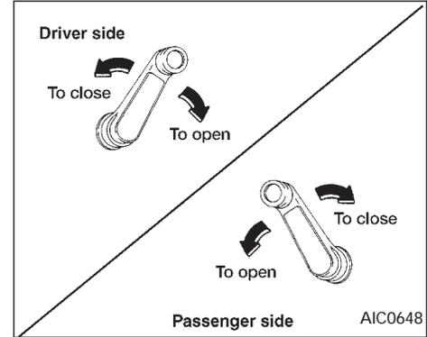
The side windows can be opened or closed by turning the hand crank on each door.
